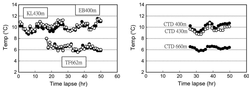
**Fig. 12** (Left) Phosphate and silicate data taken from Fig. 4 were used to calculate for the intake temperature using Eq. (7). The results from phosphate (dot) and silicate (circle) coincide with each other
