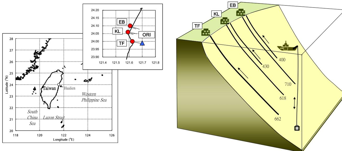
**Fig. 1** Location of deep ocean water pipelines deployed off Hualien coast, eastern Taiwan. They are operated by three factories (TF, KL, and EB). The intake points are at the far end of pipelines at depths between 400 and 710 m (also see Table 1). In this study the
