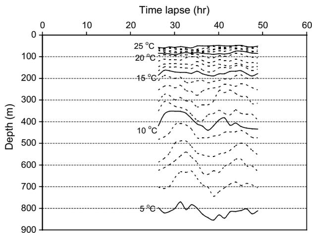
**Fig. 7** Vertical semidiurnal displacements as shown by temporal variation of isothermal lines between 25 and 5 °C. During the observed 24-h period, vertical displacements of ca. 100 m occurred below 12 °C (corresponding to deeper than 300 m layers). The time scale is the same as Fig. 4
