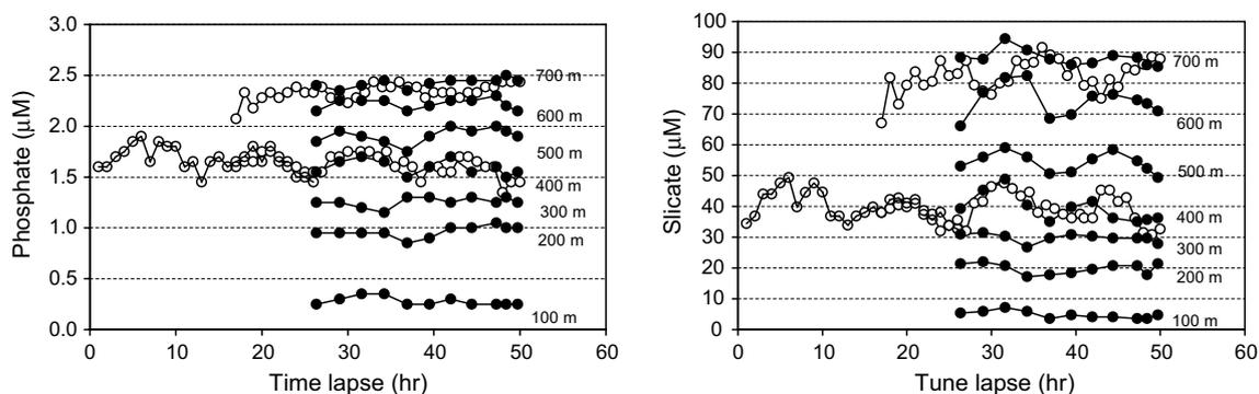
**Fig. 9** (Dots) Temporal variations of nutrients (left phosphate; right silicate) of shipboard data at different sampling depths. (Circles) Variations in nutrients in pipeline water of KL-430, EB-400, and TF662 taken from Fig. 4
