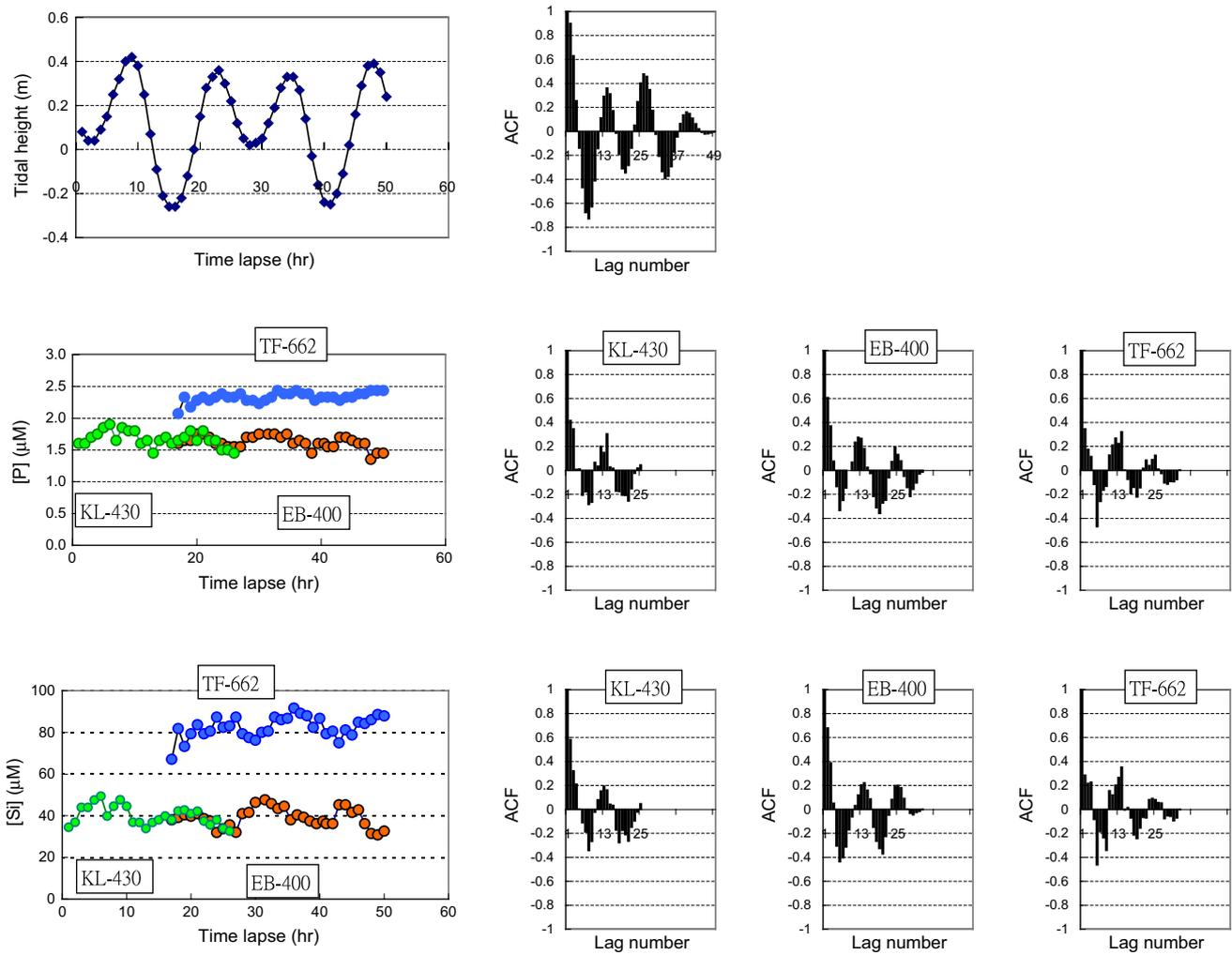
**Fig. 4** Time series plots and autocorrelation plots of (top) tidal height at Hualien (middle) phosphate and (bottom) silicate at three pipeline stations marked with their intake depths, i.e., KL-430, EB-400, and TF-662. The horizontal scale shown is the time lapse in hour-long increments beginning at 15:00, Nov 3, 2015. The correlograms are shown on the right starting from the first samples
