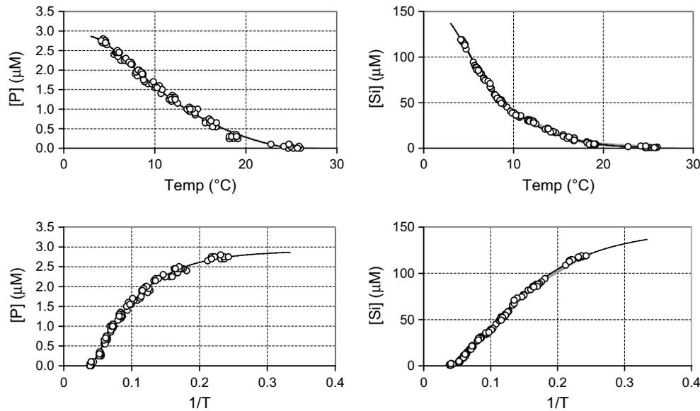
**Fig. 11** Relationships between nutrient concentrations and temperature ( $T$  and  $1/T$ ) along the water column off Hualien coast. Circles are measured nutrient data at different depths in 11 up-casts with corresponding CTD down-cast temperature data. The relationship can be
