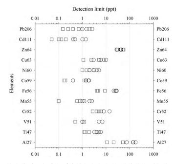
**Fig. 3.** The detection limits of Al, Cd, Co, Cr, Cu, Fe, Mn, Ni, Pb, Ti, V, and Zn. The samples include acidified Milli-Qwater (open square) or acidified chelated seawater (open circle) after being processed by the FI-IC system. The detection limits are estimated by 3 times of the standard deviation of the blank value.
